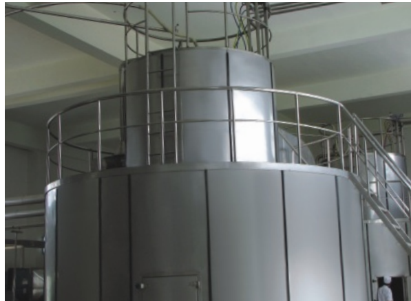
奶粉工程喷雾干燥塔顶装置 Equipment on top of the spray drying tower for milk powder
